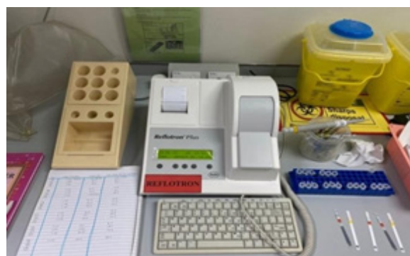
Figure 13 Estimation of plasma lipid profile using a Reflotron biochemical analyzer and lipid profile analytical strip.
