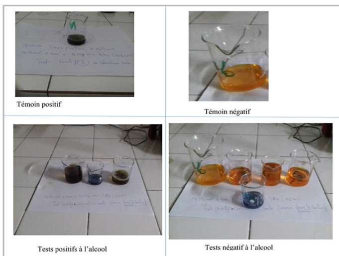
Photo 1 Colorful test with Potassium dichromate
