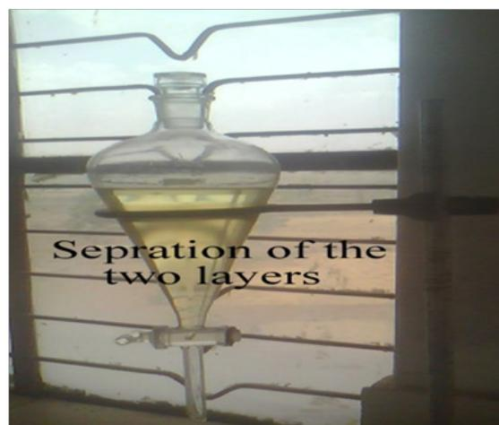
Figure 3 Separation of hexane layer.
