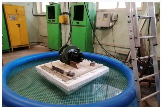
Figure 1 A test bench for researching a new principle of motion with a model of the thrust. 14
