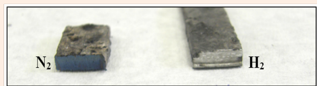
Figure 7: Coupons after plasma treatment. The nitrogen one seems to have a metallic azure colour in its cross section (nitriding).
