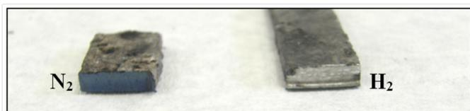
**Figure 7** Coupons after plasma treatment. The nitrogen one seems to have a metallic azure colour in its cross section (nitriding).
