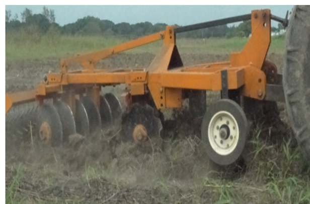
Figure 3 12-disc harrow plus lump breaker, used integrally as components used for secondary soil tillage. Drawings provided by the author, August 2021.
