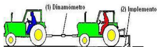
Figure 1 Pulling force of an implement coupled to the tractor.
