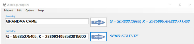
Figure 1 General view of the screen. The first row: list of possible actions, described under this Figure. The second row: the window for decoding n -block. The result is shown besides. The third row the window for encoding numbers G and K . The encoded block is shown besides. The button of action is in the middle of the rows. Some known encryptions are chosen as illustrations.
