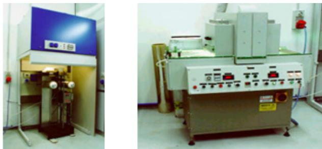
Figure 1 PDLC coater/laminator (left) and UV curing conveyor (right) systems.
