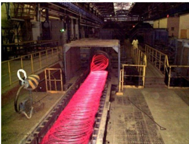
Figure 2 Shows the production process of coils rods at the wire rod mill.
