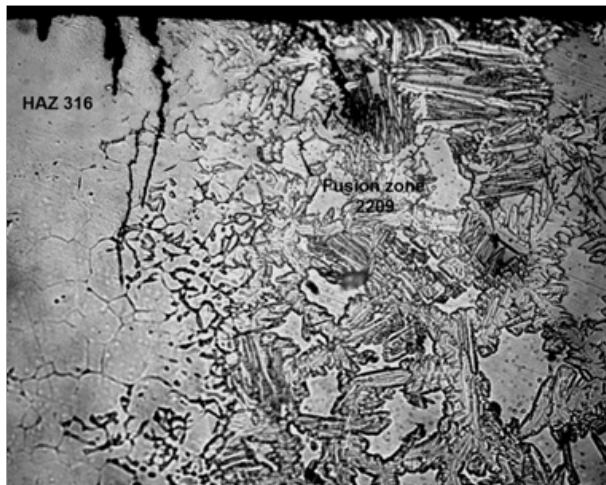
Figure 6 Microstructure of dissimilar weldment with E 2209 weld metal showing corrosion stress cracks in the HAZ on the 316 steel base metal side. Note the presence of delta ferrite network which facilitated the crack propagation.
