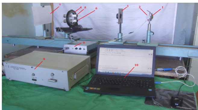
Figure 1 Photo of the laboratory desk for calibration of solar sensors.
