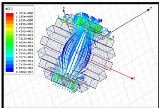
**Figure 1a)** Magnetic field induction map,  $B = (17,2 - 34,2)$  mT.
