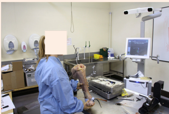
Figure 1: Set up demonstrating the rigid body markers attached to the tibia and femur and computer navigation system. Also noted is the hooks inserted in the tibia for varus and valgus stress application.
