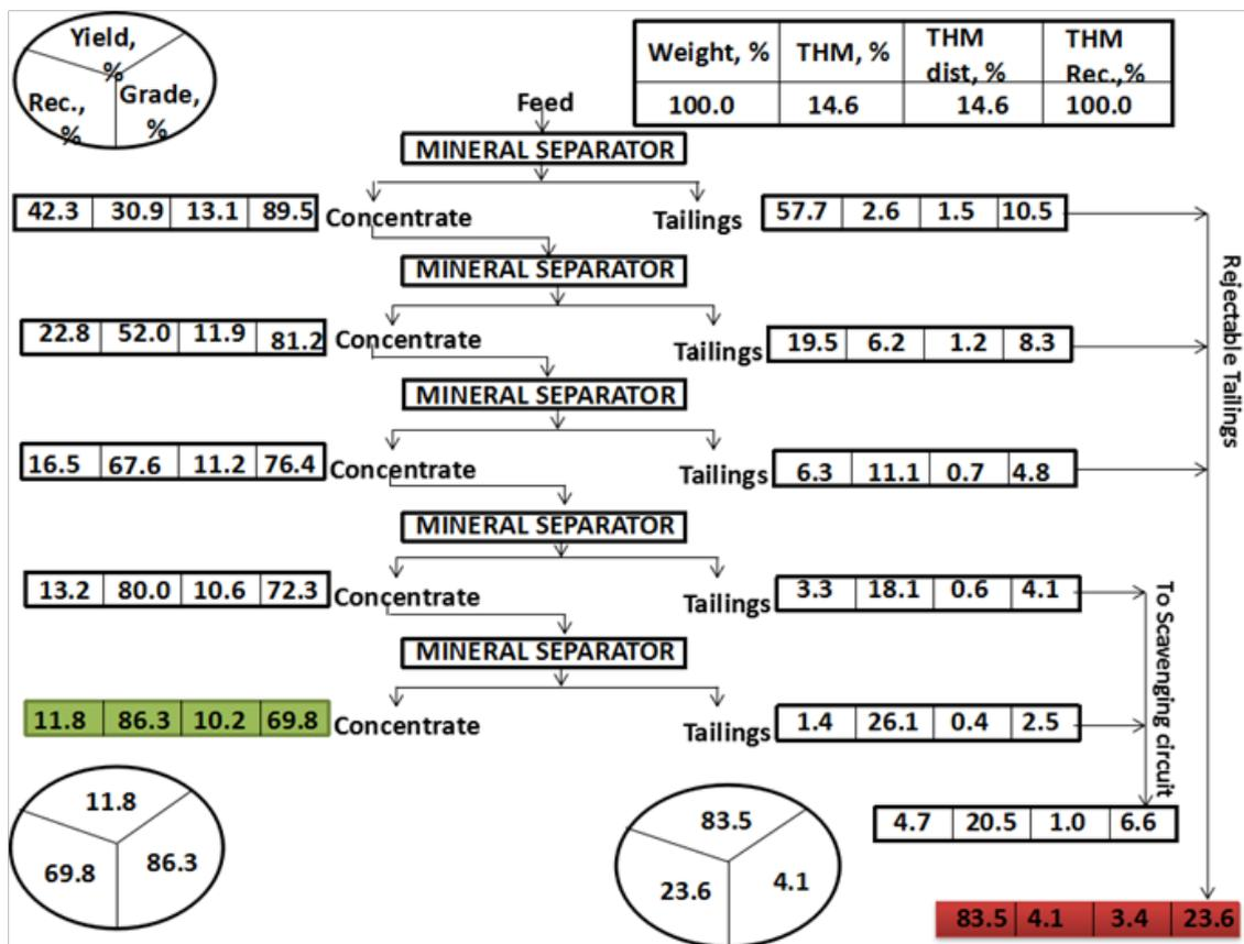
Figure 4 Flow sheet with material balance on recovery of total heavy minerals from composite sample beach –dune sand using mineral separator.
