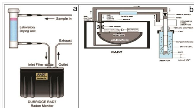
**Figure 2** A) Showing the purging process of RAD7; B) Schematic diagram of RAD H2O assembly.
