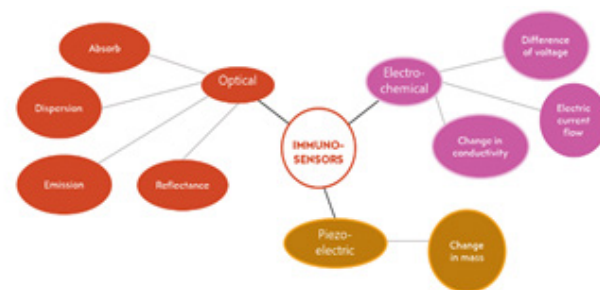
Figure 3 Types of immunosensors.
