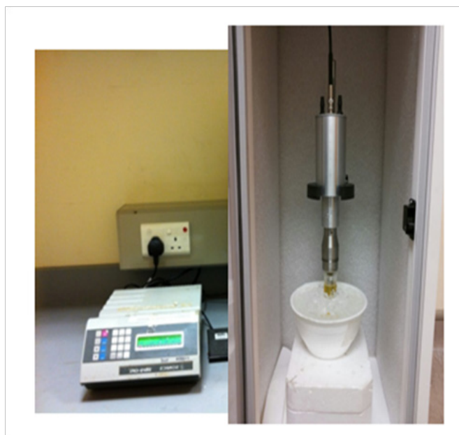
Figure 2 Ultrasonic processor with a probe horn for UAE.
