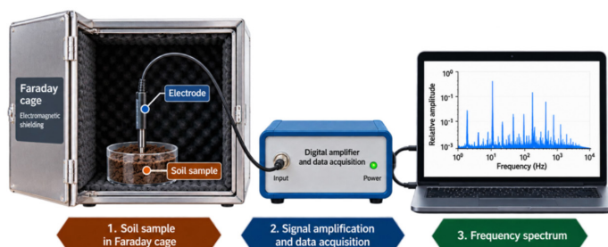
Figure 2 Graphical representation of the experimental setup for acquisition and frequency-domain analysis of spontaneous soil electrical signals.
