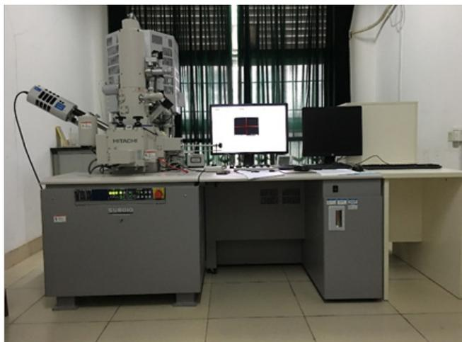
**Figure 1** SU8010 scanning electron microscope used for SEM analyses.
