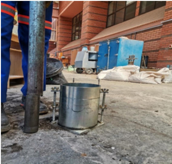
Figure 3 A picture of tamping rod and mould with a base plate.
