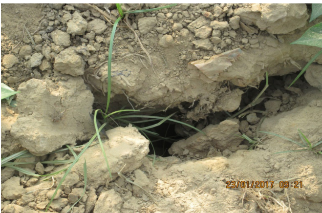
Plate 4 View of tension crack Sagbagreia.
