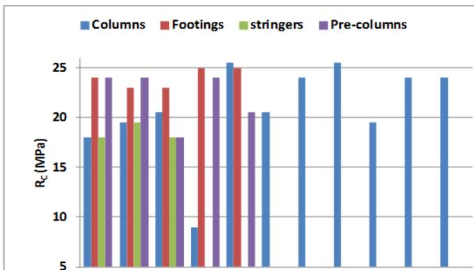
Figure 7 Compressive strength of reinforced concrete elements.
