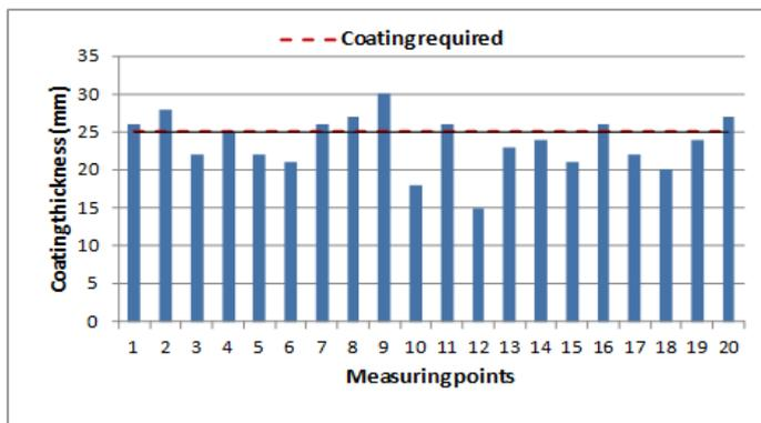
Figure 6 Measurement of the coating thickness of the concrete.
