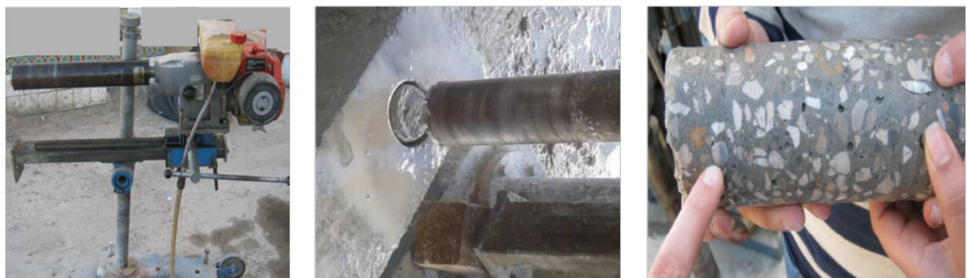
**Figure 3** Drilling operations from hardened concrete.
