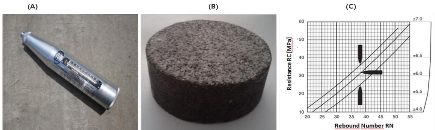
**Figure 2** Schmidt rebound hammer test
