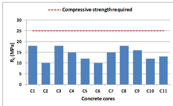
Figure 8 Compressive strength of reinforced concrete cores.
