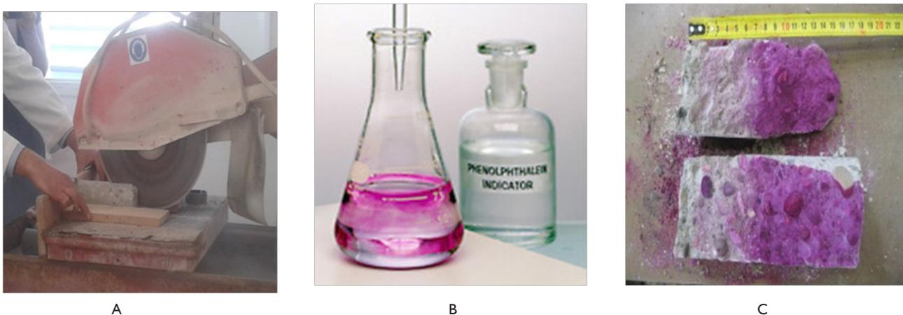
**Figure 5** Measurement of hardened concrete carbonation depth.
