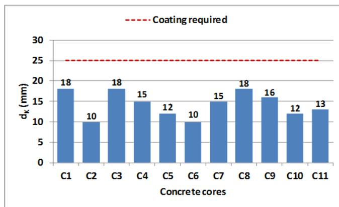
Figure 9 Hardened concrete carbonation depth of reinforced concrete cores.
