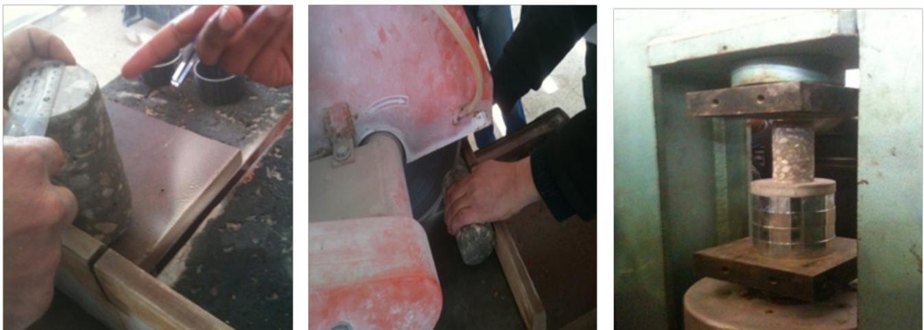
**Figure 4** Compressive strength test of core specimens.
