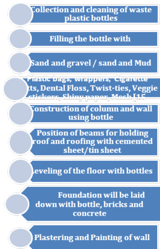
Figure 6 Methodology for construction of plastic bottle House.
