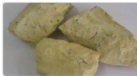
Figure 5 Samples of limestone blocks imbibed in water.
