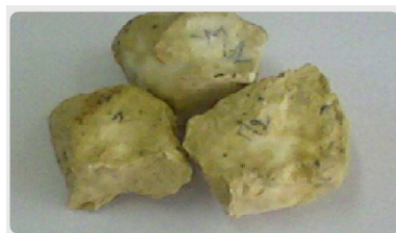
Figure 4 Samples of paraffin limestone blocks.
