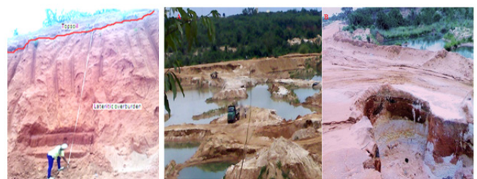
Figure 4 (A) Field measurement of pit depth and slope (Left), (B) Pit excavation causing pocket of pond (Centre) and (C) Pit excavation causing dangerous landscape, destroy access road (Right).
