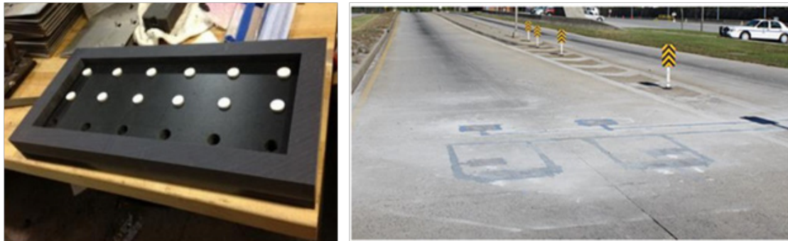
Figure 2 Piezoelectric energy harvesting system developed by Xiong. 2
