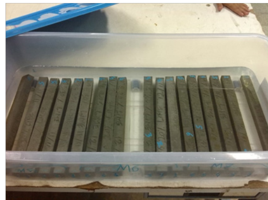
Figure 2 Mortar bars immersed in Na 2 SO 4 solution.
