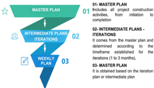
Figure 9 Application of Last Planner in time management. Elaborated by Y. Frangakis.
