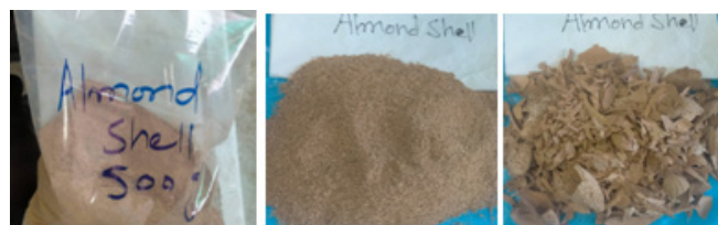
Figure 7 Sieve size of almond shell large particles on right and small on left.
