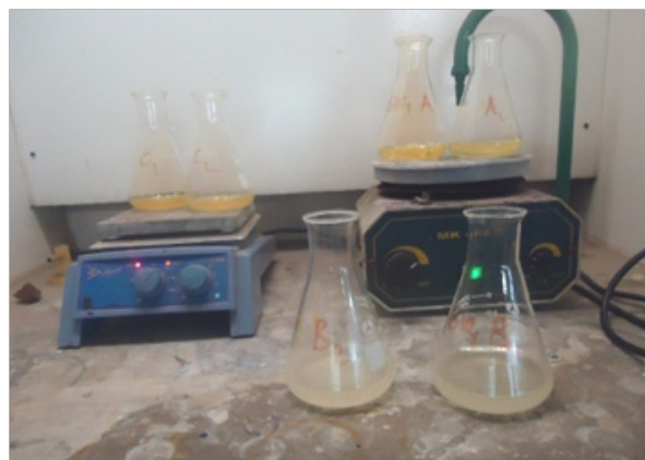
Figure 3 Sample digestions under a fume hood.
