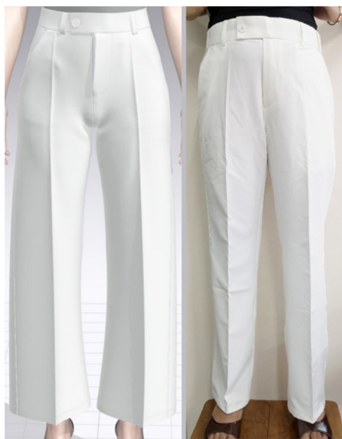
Figure 10 Comparison of drape formation between simulated and physical garments.
