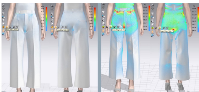
Figure 7 Strain and stress maps indicating tension distribution across the garment.
