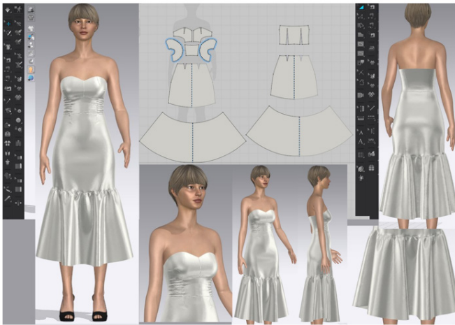
Figure 12b Flounce Simulation CLO3D simulation demonstrating how geometric Flounce application generates continuous drape, edge flow, and volumetric articulation, (Source: Author's CLO3D simulation).
