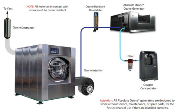
Figure 3 Ozone for Textile Application Diagram. 17
