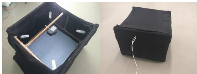
Figure 1 (a) Dark chamber with equipment fixed on the upper face and the textile sample on the lower side; (b) Dark chamber fully enclosed with external illumination.
