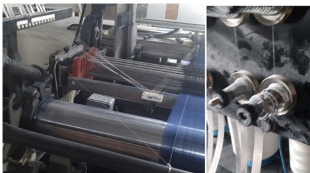
Figure 3 Arrangement of selvage yarn feeding at the weaving machine and defective spring tensioners which were removed.
