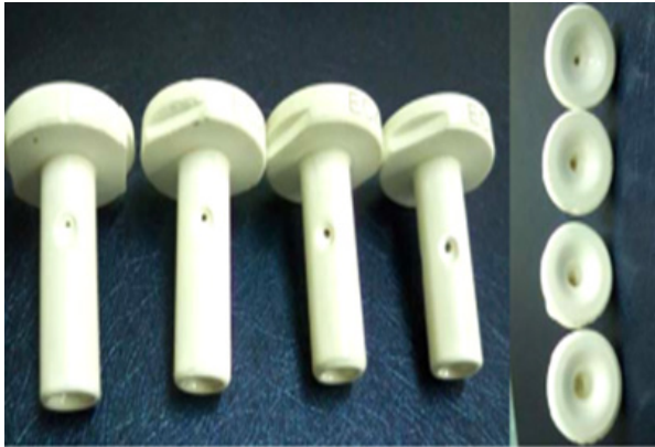
Figure 3 The real views of the single jet (nozzle) used in ATY yarn production. 8
