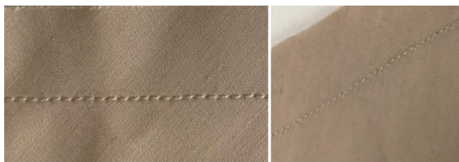
a) Two-thread lock stitched test sample
