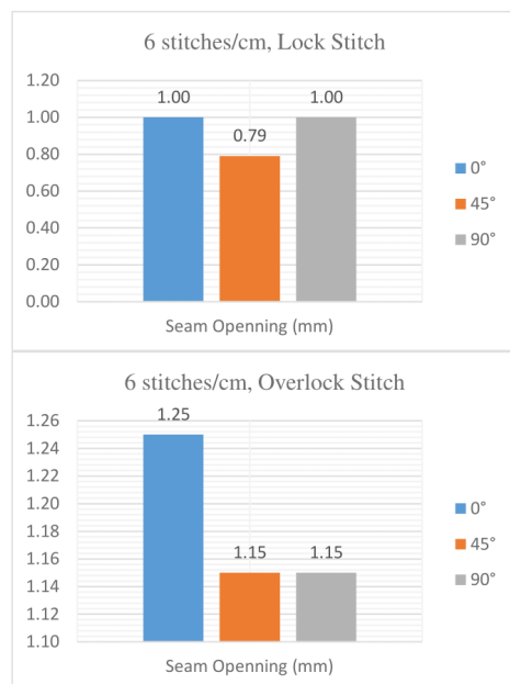
Figure 9 Seam slippage results at different sewing directions, 6 stitches/cm, a) lock stitch b) overlock stitch.
