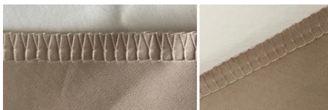
b) Four-thread overlock stitched test sample
