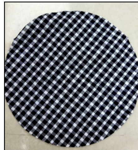
Figure 2 Weight (g/m 2 ) measurement of the fabric.
