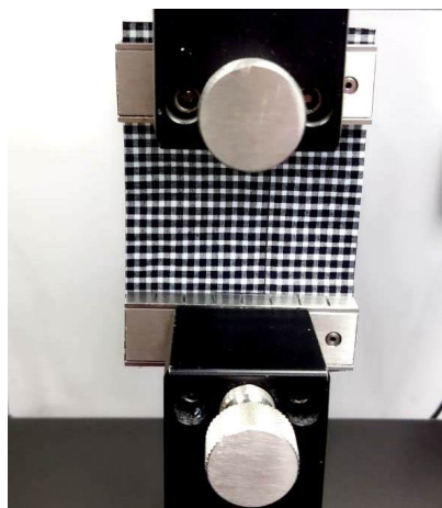
Figure 4 Tensile strength measurement process of fabrics.
