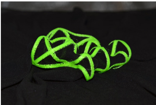
Figure 11 Key point of self-forming was to establish closed pattern to print.
