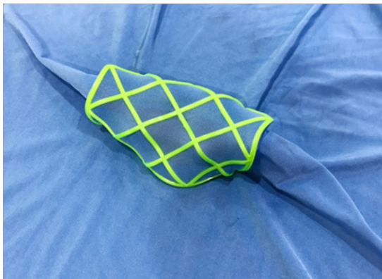
Figure 10 The larger elastic the small-meshed fabric was, the greater deformation.
