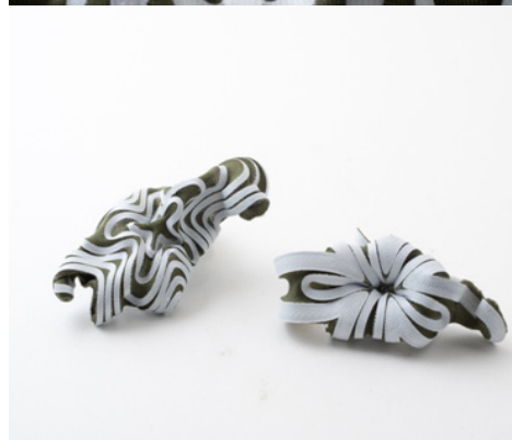
Figure 6 Plastic patterns inhibited the contraction of the surface, guiding the stretched fabric to gain its desired shape.
