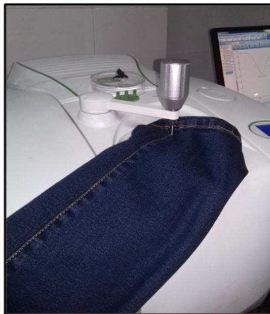
Figure 6 FTIR experiments of woven garments.
