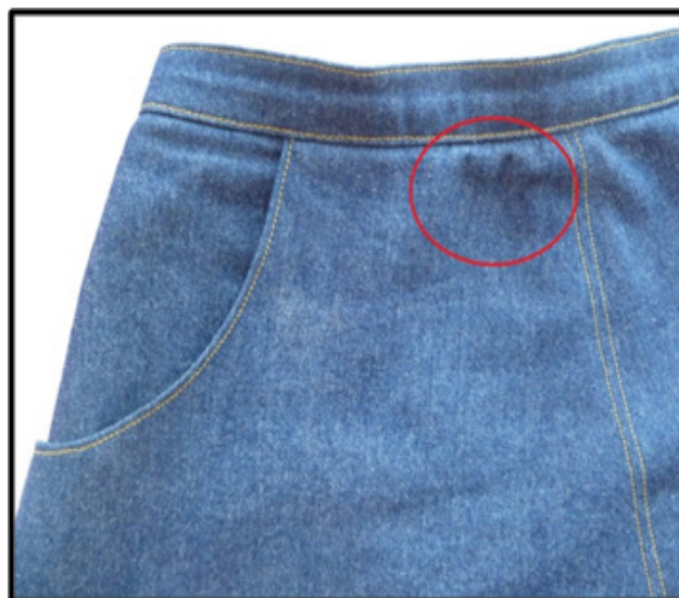
Figure 4 Spandex damage in the fabric.
