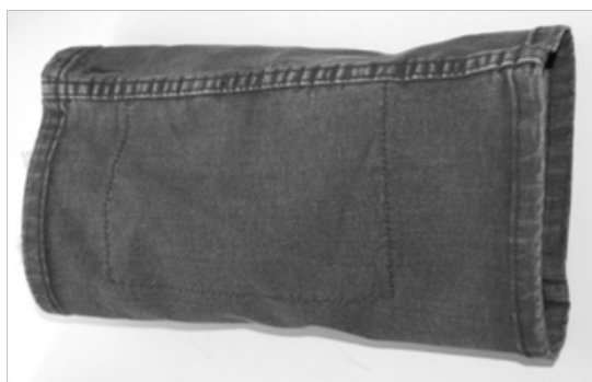
Figure 1 Leg panel for the washing trials. The stitch shows the pocket fabric inside the leg panel.
