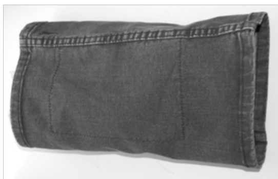
Figure 1 Leg panel for the washing trials. The stich shows the pocket fabric inside the leg panel.
