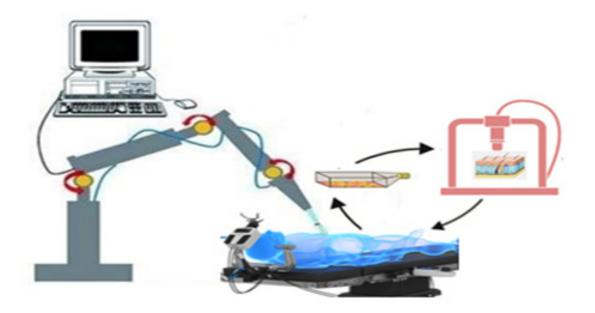
Figure I Robot-aided 3D bioprinting. Diagram explains the notion of robot-aided in vivo 3D bioprinting in the cadre of minimally invasive surgery.
