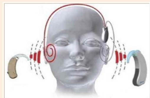
Figure 3: Scheme demonstrating the sounds captured by the microphone of the speech processor and the conventional contralateral microphone connected to it. Both are processed by the speech and sent to a single implanted receiver-stimulator, responsible for transmitting information to both beams ipsilateral and contralateral electrodes processor, so that they promote synchronous pacing in the remaining nerve fibers in both cochlea.
