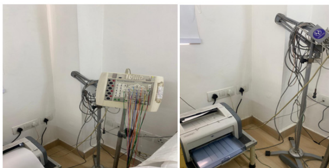
Figure 2 The image portrays potential source of power fluctuations in a hospital room. The EEG machine is positioned next to a printer. Both devices are plugged into the same power outlet. This setup can introduce electrical noise into the EEG signal. In clinical settings, dedicated outlets or surge protectors are recommended to minimize interference and ensure reliable EEG recordings.
