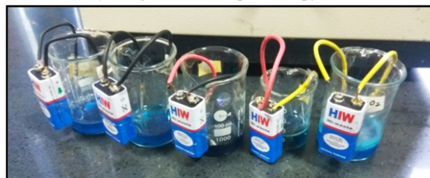
Figure 1 Photograph of as constructed photo reactive system for degradation of MB dye.
