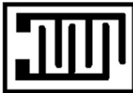
Figure 2 Glass substrate with inter digitated electrodes for making gas sensor.
