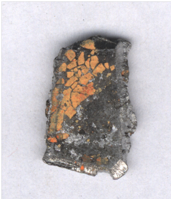
Figure 1 A piece of pewter alloyed by the author. The orange litharge is markedly visible.
