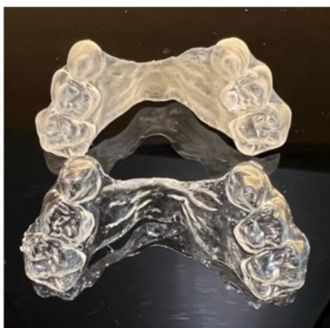
Figure 4 Above, Expander 1, for which the post-curing process was delayed by 12 hours. Transparency was severely impacted compared to Expander 2, where the process followed the manufacturer's recommendations.
