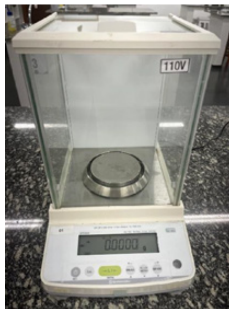
Figure 7 High-precision digital analytical balance with BEL® glass container.
