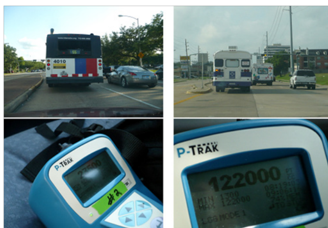
Figure 7 UFP monitor readings while following vehicles emitting excessive exhaust.
